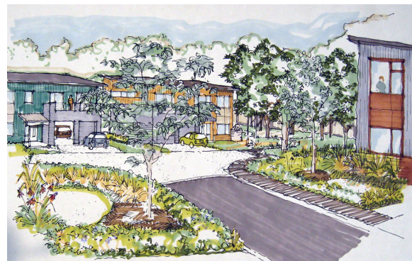
Figure 8-16. Conceptual drawing of Tonbo Meadow hammerhead turnaround designed to use porous pavement (courtesy of Lara Berkley, ASLA, and Scott Ogden, AIA, of B+O Design Studio, PLLC)
