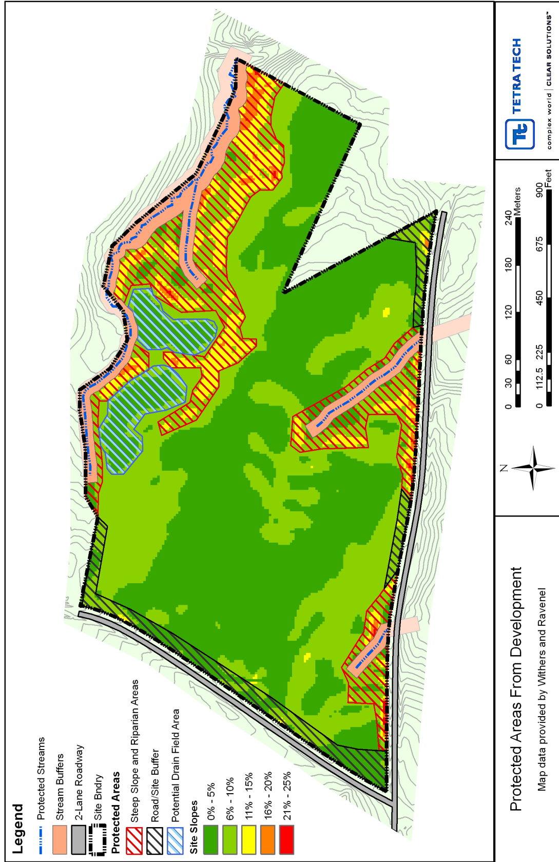
Figure 8-32. Desired areas for protection from development
