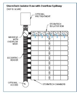
If upon visual inspection it is found that sediment has accumulated, a stadia rod should be inserted to determine the depth of sediment. When the average depth of sediment exceeds 3 inches throughout the length of the Isolator Row, clean out should be performed.
