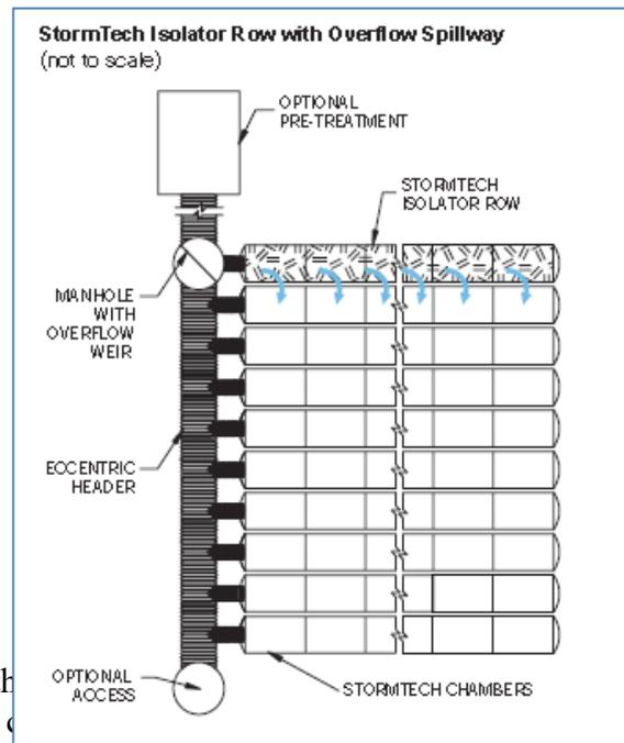
If upon visual inspection it is found that sediment has accumulated, a stadia rod should be inserted to determine the depth of sediment. When the average depth of sediment exceeds 3 inches throughout the length of the Isolator Row, clean out should be performed.
