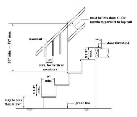
FIGURE 3.11 Stair and Rail Geometry
