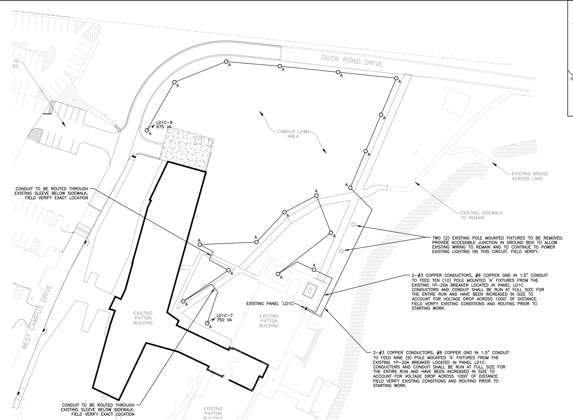
1 PARTIAL SITE PLAN – LIGHTING (BASE BID)  $\sqrt{E101/SCALE: 1" = 40'-0"}$
