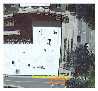
Vehicle Parking for 1 Contractor Truck. Drawing show what appears to be 4" thick concrete. Contractor may park (1) pickup truck here, but he will be responsible to repair any concrete that cracks from using this for parking. He must also provide and use protective matting to protect the concrete and provide a barricaded pedestrian path on both sidewalks.
