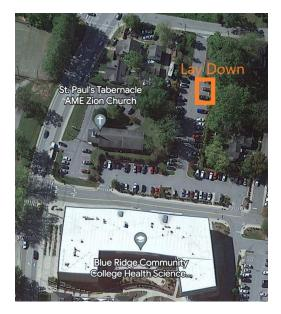
Parking for Concrete Truck, Dump Truck for concrete debris & Pumper for Concrete. Contractor must provide cones and traffic control 1 lane closure. 1 lane must stay open at all times. Contractor should make every effort to provide pedestrian pathway when transporting concrete debris down the sidewalk from the steps to the loading zone.
