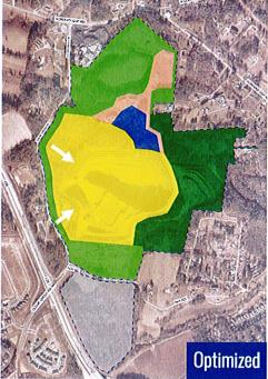
Operations Area Mining Area Overburden Area Stockpile & Customer Loading Plant Area
