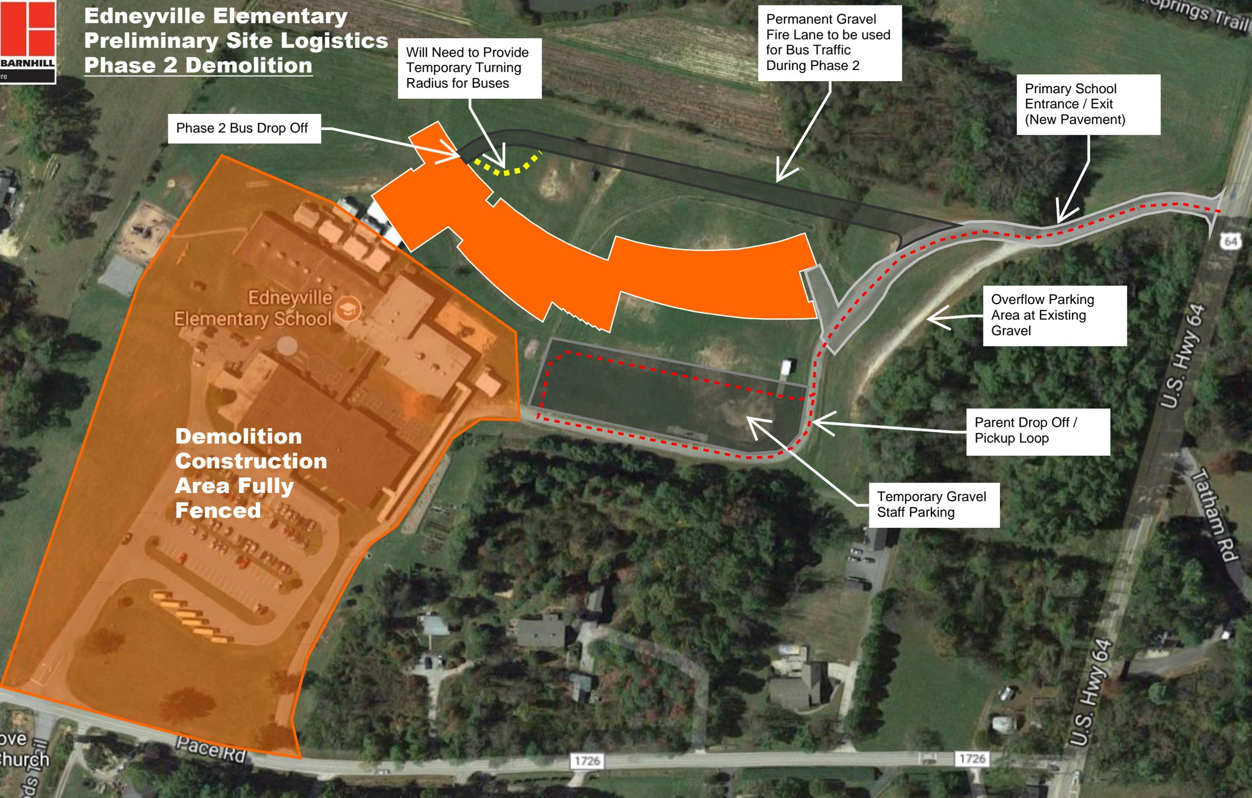
Will Need to Provide Temporary Turning Radius for Buses
