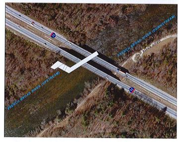
The final causeway will be used to remove the center bars of bridge.
